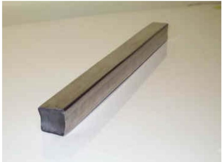
1.25 Inch square bar (Above) was produced from a plasma cut rectangle and cold rolled 45%. Hardness is Rockwell C 40, and the Ultimate Tensile Strength is over 200 KSI.
